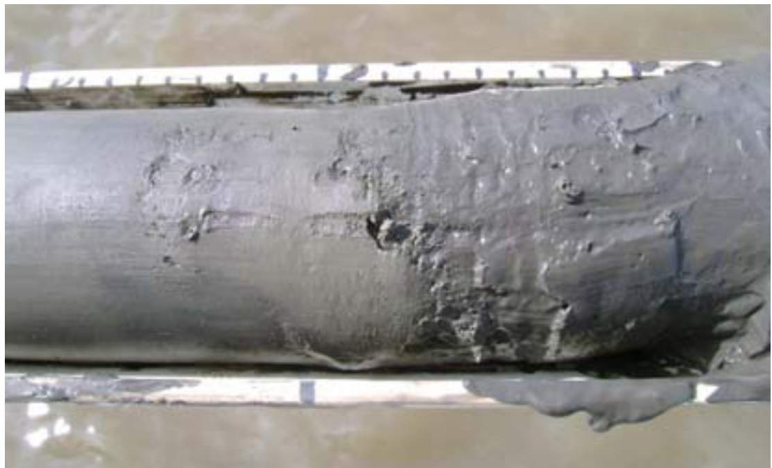
Figure 3. Sediment core from Mission Lake in Brown County, Kansas, showing pre-impoundment substrate (left) and post-impoundment sediment (right) Photo courtesy of Kansas Biological Survey
